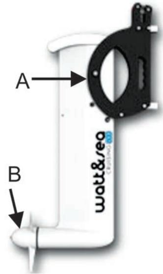
Figure 2: "A" is a fixed unit mounted on the transom that can be swung down into the water. "B" is the propeller that is mounted directly to the sealed generator.
