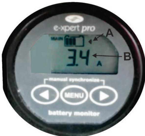
Fig. 3: Shows the Regen on our electric conversion Yamaha 33 sailboat while under sail at just over 5 knots. "A" is an arrow that points toward the battery symbol when charging is going on. "B" shows the amount of charging that is going on- in this case, 3.4 amperes plus .5 amperes that the system is using.
