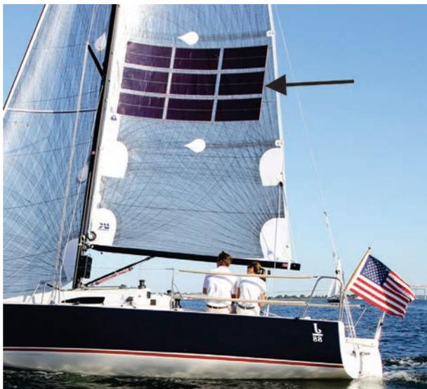
Figure 1: Solar panels sewn or laminated into the mainsail. The arrow indicates the three rows of panels.
