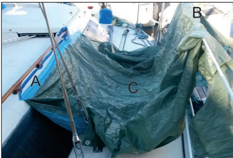
Figure 1: Preparing to remove the old varnish, we taped, "A", the tarp in place and then laid it over the lifelines, "B", to create a trough, "C", that will keep everything out of the water. We are doing this one section at a time.
