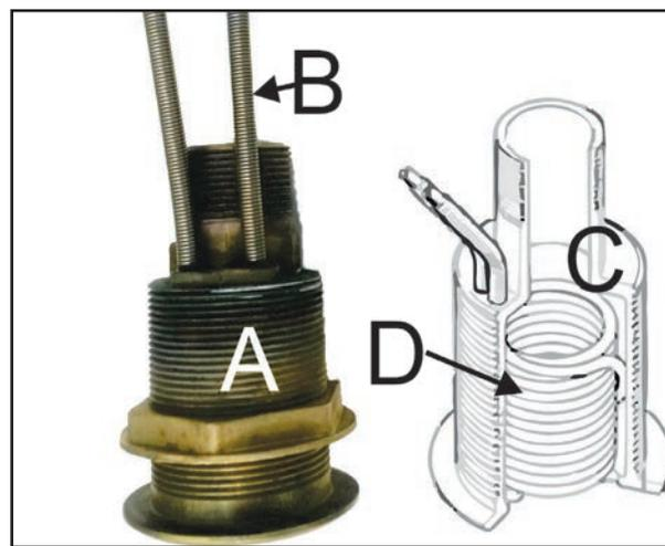
Figure 3: "A" is a special thru-hull fitting, used effectively to water cool some refrigeration systems, that is constructed with coils inside that exit at the top, "B." "C" is a cutaway drawing of the same thru-hull fitting that shows the coils, "D."
