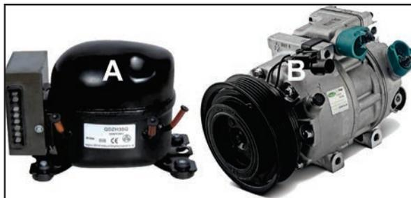
Figure 2: "A" is a sealed electric refrigeration compressor that can run either on 12 - 24 volts DC or 120 volts AC. This is usually paired with an evaporator. "B" is an open, belt-driven refrigeration compressor that can be mounted on the main engine or the generator. It is normally connected to a holding plate.
