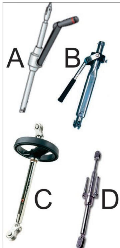
Figure 2: Mechanical backstay adjusters come in many configurations: "A" uses a winch handle to get you plenty of leverage, and, then, when the handle is removed, you have a snag free backstay. "B" has a ratcheting handle that tucks out of the way. In "C" the wheel is snag free, but the length of the mechanical advantage is less than some others. "D" has two folding handles that are not much longer than that of "C". They all aim for snag free mechanical advantage.
