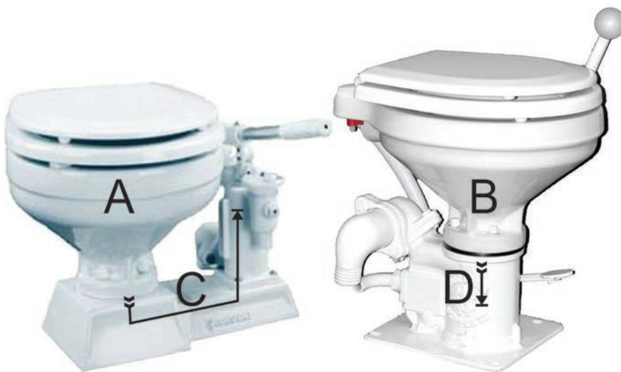
Figure 1: "A" is a side-mounted piston pump plastic toilet and "C" is just above the arrowed line indicating the pump suction direction. "B" is an in-line, bronze piston pump toilet, and "D" is next to the arrowed line indicating its direction. Note the difference in the intake distance to the piston.
