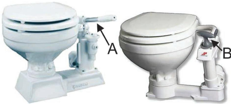
Figure 2: These two toilets are side-mount piston pump style, but "A" indicates the lever that will make it easier to pump. "B" has a handle screwed to the end of the piston rod with no mechanical advantage.
