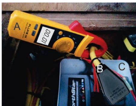
Fig. 3: This clamp on multimeter "A" is attached to the ground cable "B" of this battery bank "C". With all the devices turned off it indicates an unexplained current drain which should now be investigated.
