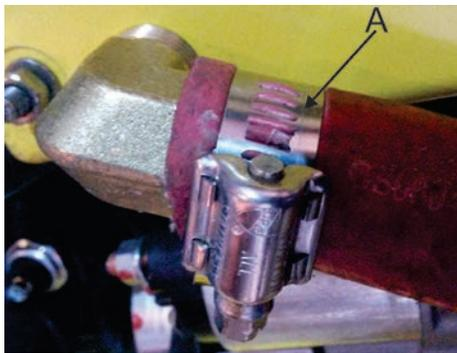
Figure 2: Automotive hose clamps like "A" are perforated through the band where the gear (screw) tightens the clamp. This causes the hose to be cut and forced into these openings thereby degrading the hose. These clamps are not 316 SS and are often welded. For this reason, they should be dismantled for inspection periodically.
