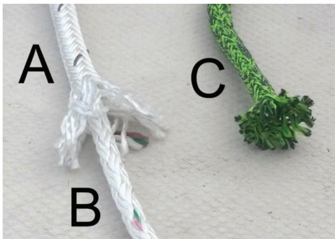
Figure 1: "A" is double braid polyester, and "B" is the core that is being extracted so the cover can be pulled over and sewn onto a Dyneema 12 strand single-braided rope. "C" is a cover that is sold for the same purpose that usually costs more than twice the double braid. As you pull the core out of the "A", you can pull the Dyneema in.
