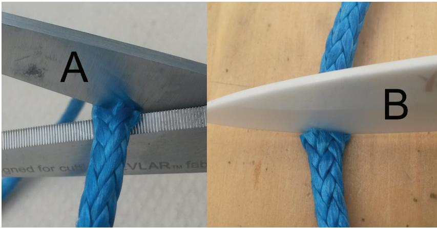
Fig. 3: "A" is a pair of scissors designed to cut Kevlar, but they work well on HMPE. "B" shows a ceramic knife that also holds an edge while cutting through HMPE fiber.
